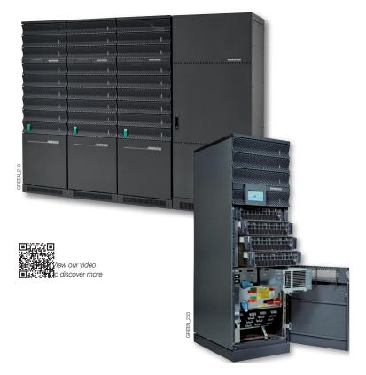
With its flexible modularity providing seamless and risk-free power scalability up to 600 kW, the MODULYS GP range is the ideal solution for unscheduled site upgrades or incremental power evolutions. The installed power can be increased up to 600 kW by adding hot-swap plug-in power modules for incremental steps of 25 kW.
